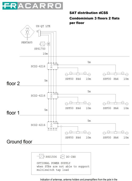
Indication of antennas, antenna holders and preamplifiers from the pole in the scheme is purely indicative, as the choice depends exclusively from the type of TV signal received in the zone of construction of the plant and the structure of the building The present scheme ofproposed maximum does not constitute a project to be drafted by designer enabled stable. The present scheme of maximum proposed does not constitutes a project that must be drawn up by a qualified designer.
